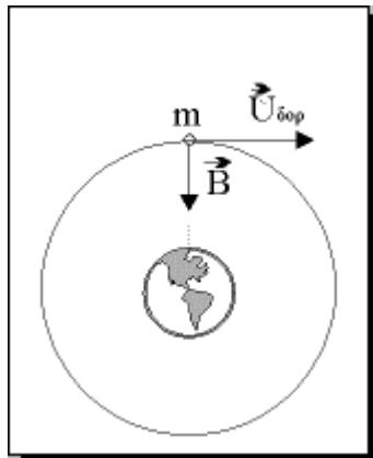
$$B = m \cdot \frac{v_{\delta\phi}^2}{r} \Rightarrow G \cdot \frac{M_\Gamma m}{r^2} = \frac{mv_{\delta\phi}^2}{r} \Rightarrow v_{\delta\phi} = \sqrt{\frac{GM_\Gamma}{r}} \Rightarrow v_{\delta\phi} = \sqrt{\frac{g_0 R_\Gamma^2}{4R_\Gamma}} \Rightarrow$$
